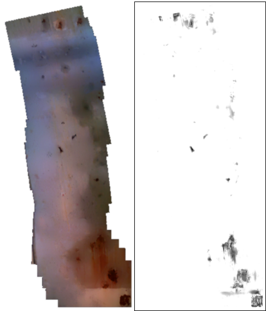
Fig. 3. Mosaic obtained after a flight and saliency-based defect detection.
