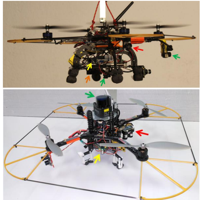
Figure 1. [top] A Hummingbird platform featuring optical flow sensors (green), an infrared height-meter (orange), and ultrasound sensors (red). [bottom] A Pelican platform featuring a laser scanner (green) and a laser-based height-meter (red). The embedded PC is indicated by a yellow arrow in each case.
