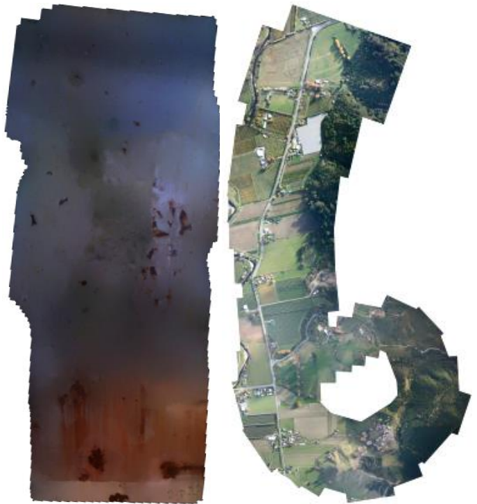
Figure 6. Mosaics from sequences resulting from an inspection operation (left) and a flight at high altitude (right).
