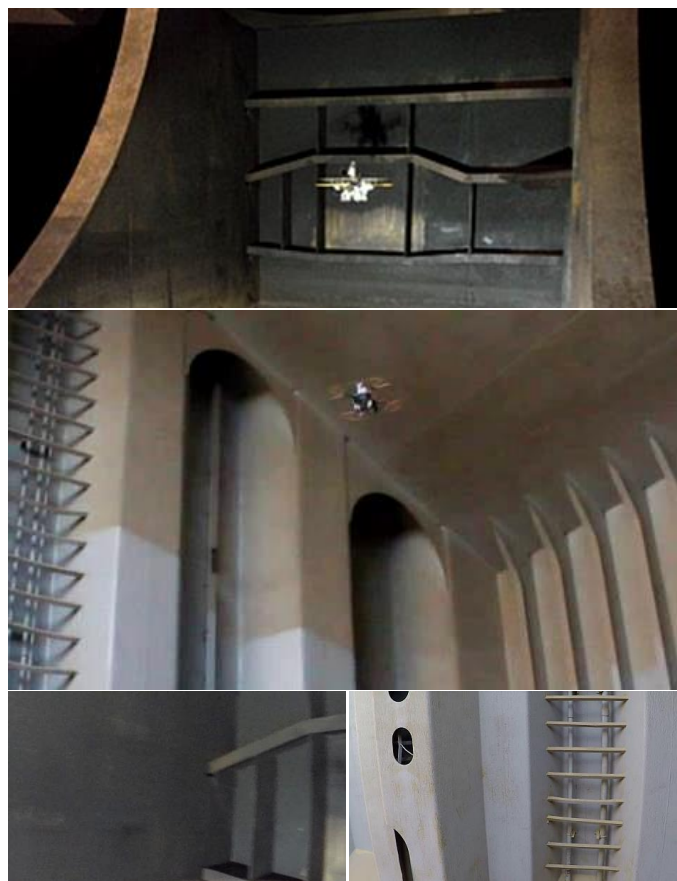
Figure 4. Visual inspections onboard an oil tanker [top and bottom left] and onboard a bulk carrier [middle and bottom right].
