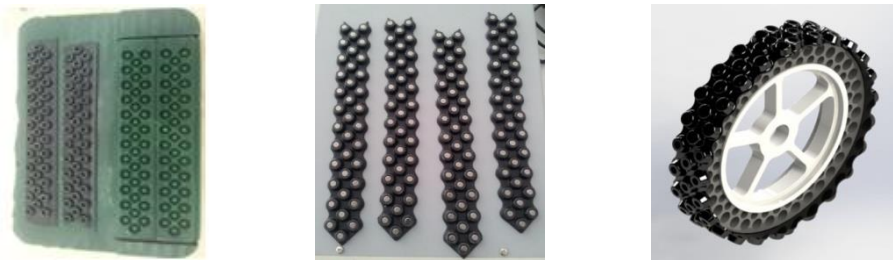
Fig. 4: Wax mould with the casted polyurethane stripes (left). Polyurethane stripes with integrated magnets (middle). Wheel-CAD model (right) (source: DFKI GmbH)
