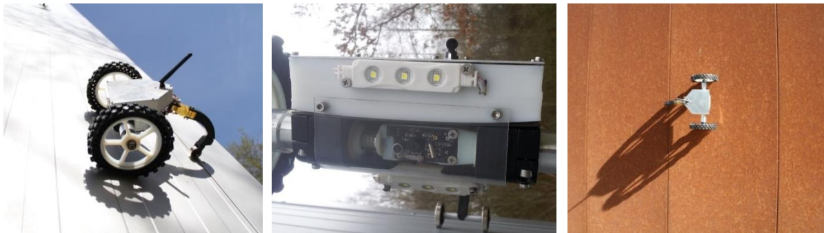
Fig. 3: The lightweight magnetic crawler. (source: DFKI GmbH)
