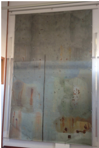
Fig. 3. Canvas used in our experiments for simulating a cargo hold wall.
