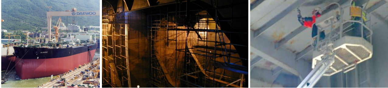
Figure 1: Illustration of traditional inspection methods: (left) general cargo ship, (center) staging previous to inspection, and (right) cherry-picking. [Source: (left,center) Lloyd's Register, (right) http://www.standard-club.com ]
