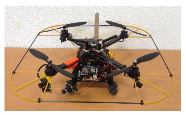
Fig. 1. The Hummingbird platform fitted with the sensor suite intended for the inspection application.
