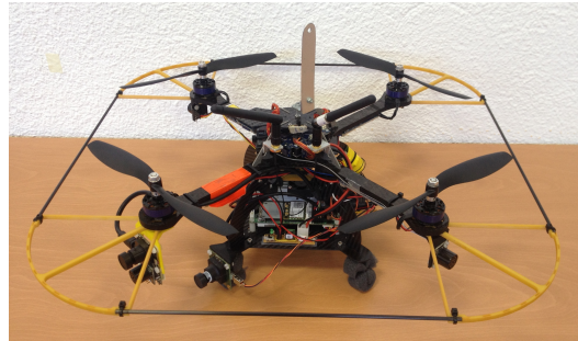
Fig. 1. The Hummingbird platform fitted with the sensor suite intended for the inspection application.
