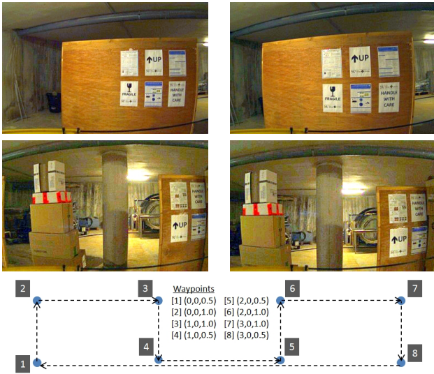
Fig. 10. Pairs of images taken at the same location in two different executions of the last experiment. The slight deviations in viewpoint are due to the orientation accuracy parameter, set to 6 degrees in the mission specification file. The drawing at the bottom shows the positions where the photos are to be taken during the inspection mission. The pairs above correspond to, respectively, locations 2, 4 and 6.
