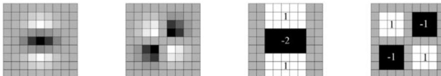
Figure 4: Left to right: the Gaussian second order partial derivatives in  $y$ -direction and  $xy$ -direction, and SURF approximations using box filters. The gray regions are equal to zero.
