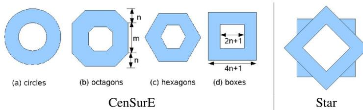
Figure 7: Bi-level filters used by CenSurE and Star
