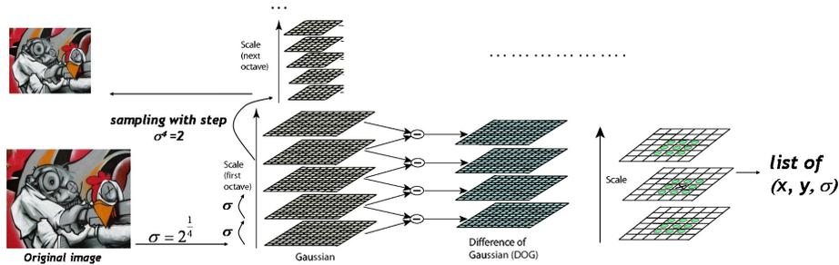
Figure 3: Overview of the DoG scheme, used by SIFT for the key point detection.
